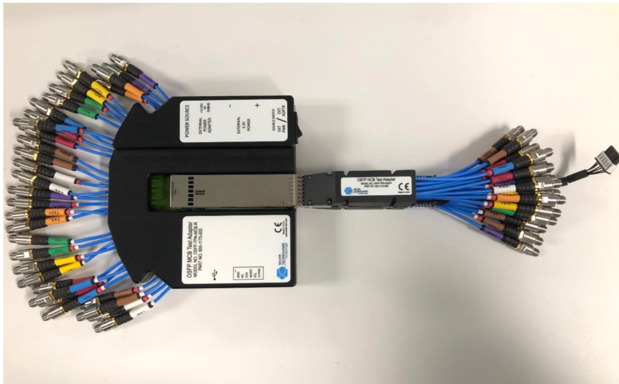
Wilder OSFP 112G mated Module Compliance Board (MCB) / Host Compliance Board (HCB)
